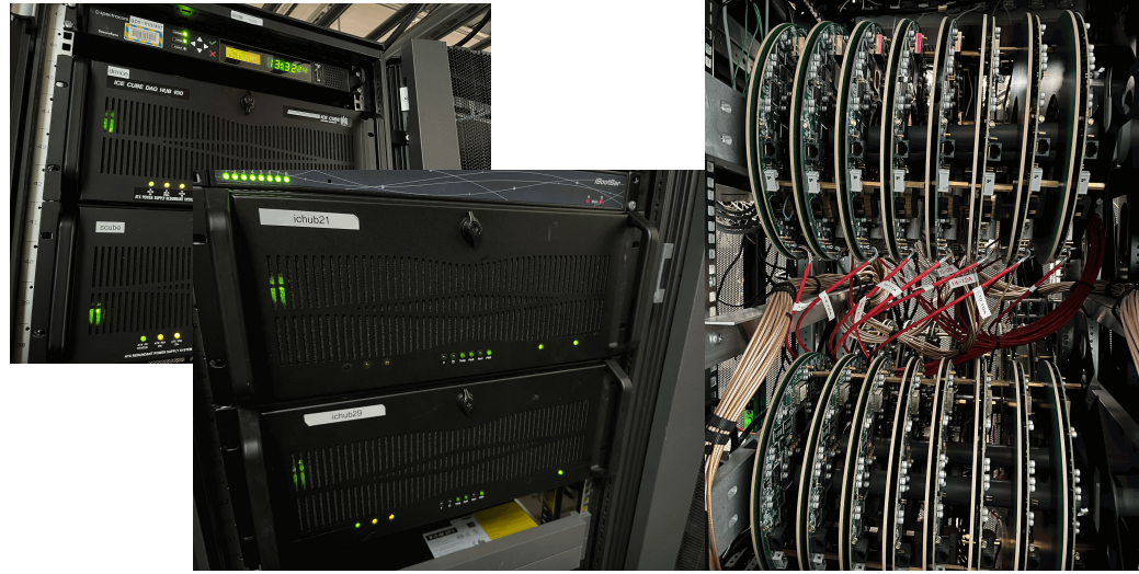
SPTS test setup - computers, “string” of DOM mainboards
